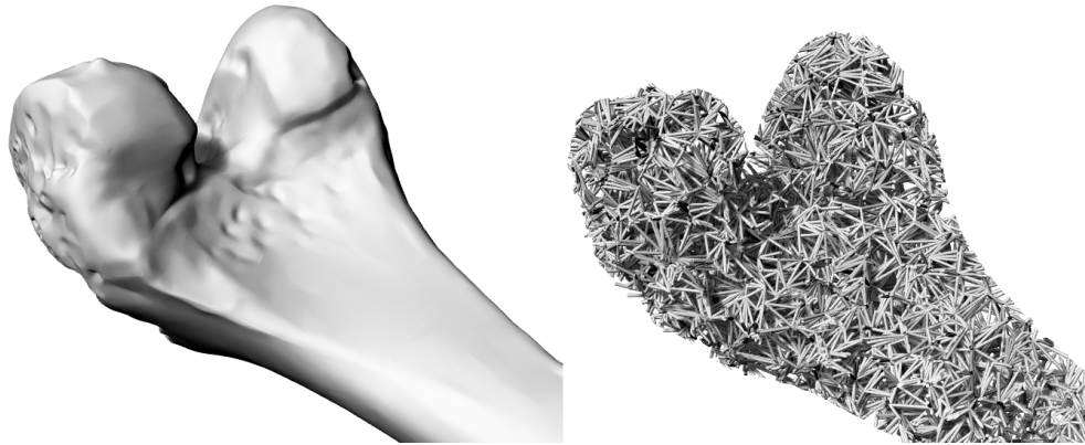
Figure 4.11 A stochastic Voronoi infill of a human femur bone
