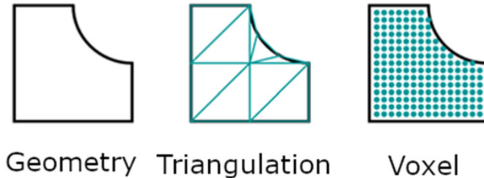
Figure 2.8 Triangular mesh and voxel methods for representing original geometry representations. Adapted from (Schnös et al., 2021).
